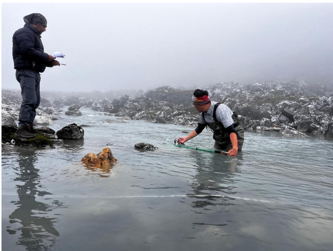
Discharge measurement in BhaleyPokhari using float method
