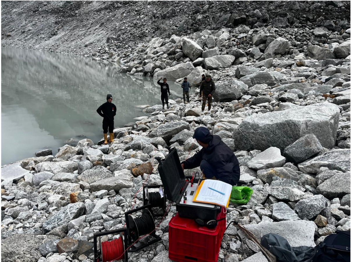
Team performing ERT survey of Tikip Lake to assess moraine stability
